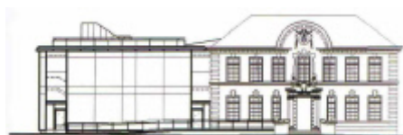
Updated south elevation showing reduced bulk of rooftop plant enclosures, panel jointing to new stonework, new ramp and planting bed
